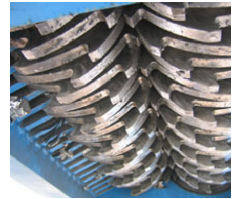
Shredding chamber discharge side shows rugged cutters
